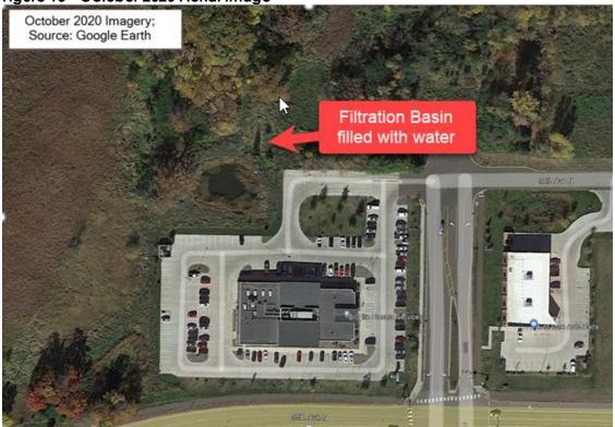
Figure 14 Standing Water in Filtration Basin Observed by City Staff in September 2021
