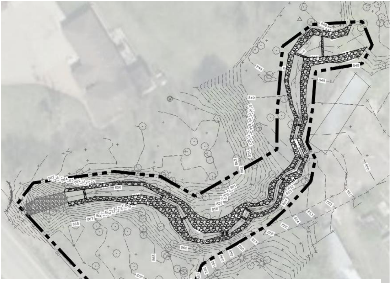
30% design showing stabilized channel and rock grade control structures
